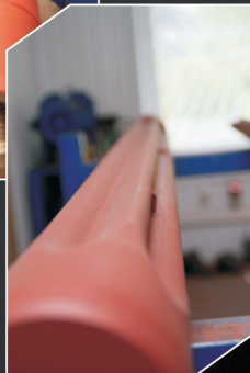
Anchor is made from profiled pipe. The length is 3-4 m
