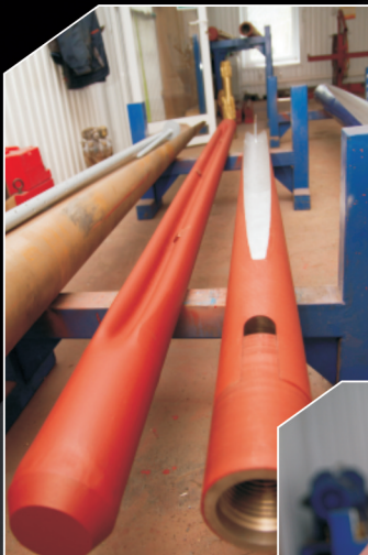
Anchor is made from profiled pipe. The length is 3-4 m
